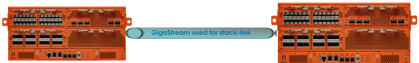
Figure 4 Daisy-Chain Configuration using GigaStream for Stack-link
